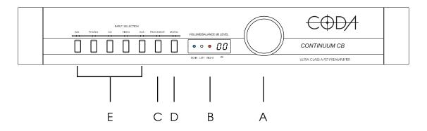
**A**: The rotary controller adjusts the currently selected volume level. Press the knob to switch between the volume setting for left, right or both channels, indicated by the lights underneath the digit display.
