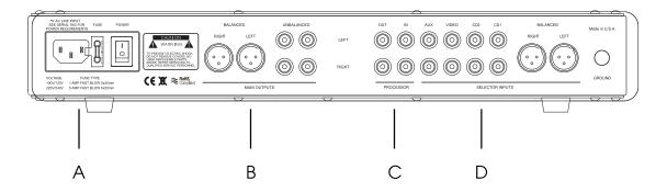
**A**: The AC receptacle accepts any standard three-prong IEC line cord. Power input can be adjusted for any country, but is set internally at the factory. Contact Coda or your local Coda dealer if the voltage must be changed. Fuse specifications are listed below the receptacle, and the fuse can be changed by unplugging the line cord, pulling out the fuse drawer and clipping in a new fuse.
